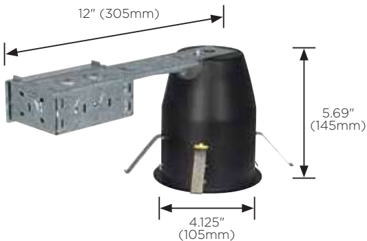
S9539 4" Can - Remodel For 120V, 60Hz, 18W max. Suitable for wet and damp locations* For use only with UL or cUL classified LED or equivalent IC Rated
